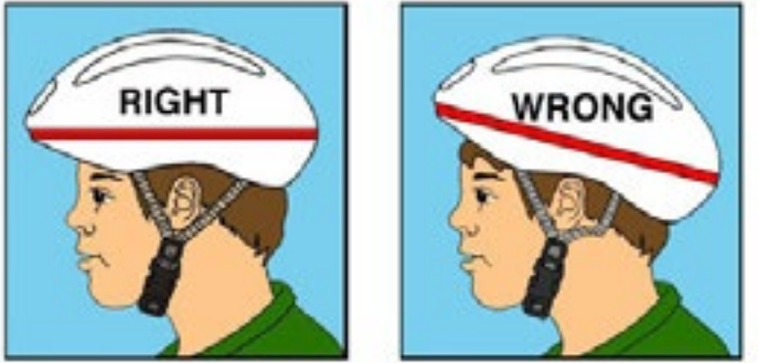
Wear the helmet flat on the head, not tilted back at an angle!
